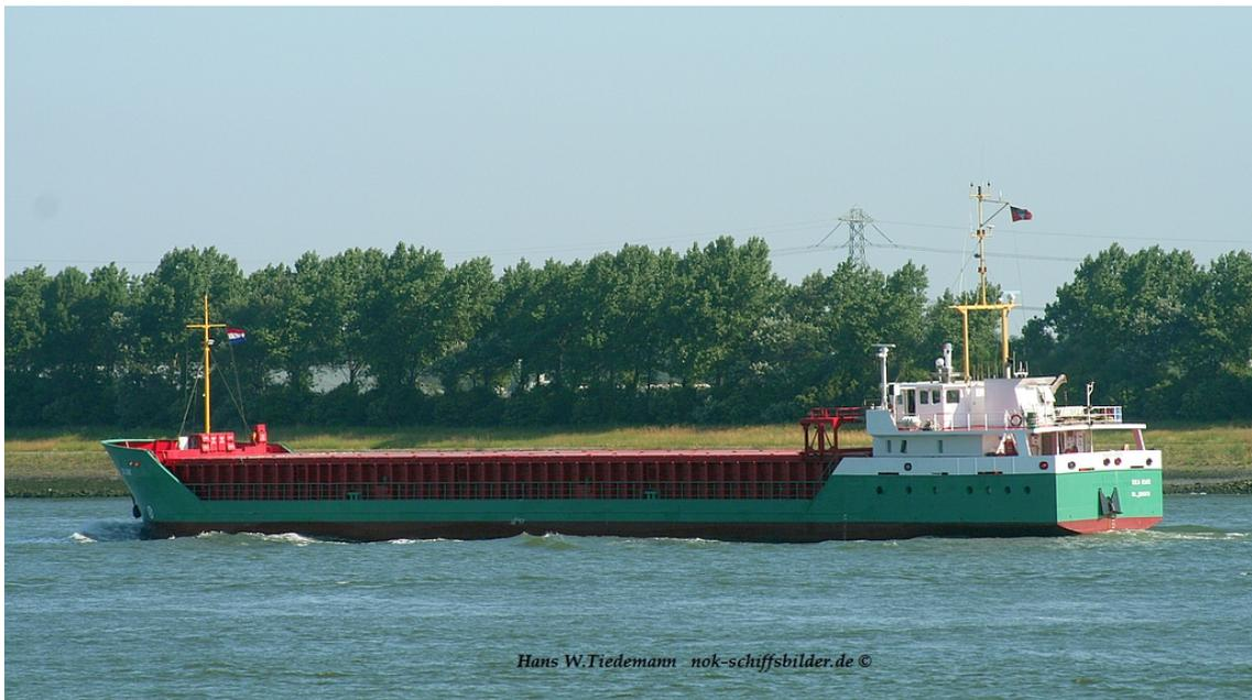
Als SEA EMS vor Rotterdam am 16.07.06 |GT :1682|DWT :2503|NT:957|Length opa:82 m|Breadth:11 m|Depth:5.67 m|Draught:4.45 m| Main Engine: 6 Cyl. MaK/1020 kW/ 10.5 kn|Year of build :1996| Builder/ Place: Veka Shipyard Lemmer B.V./Wartena (NLD)|Yard No:675
